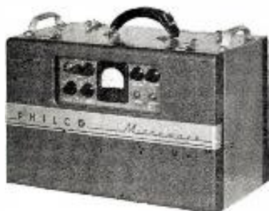
Transmitter Control and Power Supply
